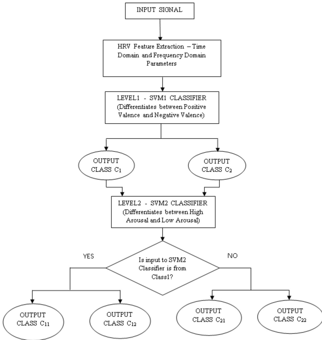
Figure 4: Multilayered SVM Binary Tree
