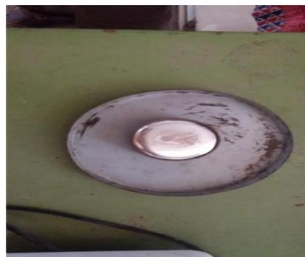
Fig. 6 Determination of Shrinkage Limit
