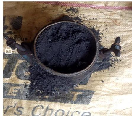
Fig. 7 Determination of OMC & MDD
