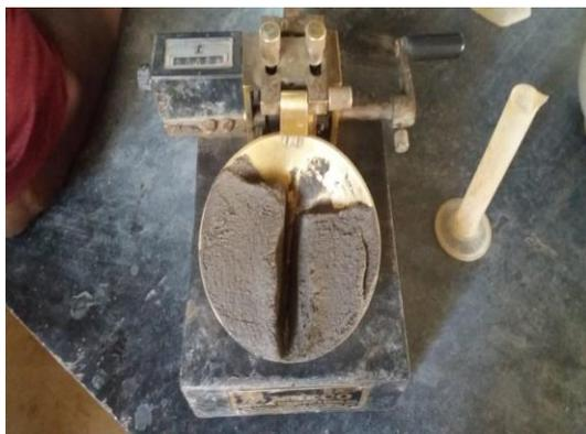
Fig. 4 Determination of Liquid Limit
