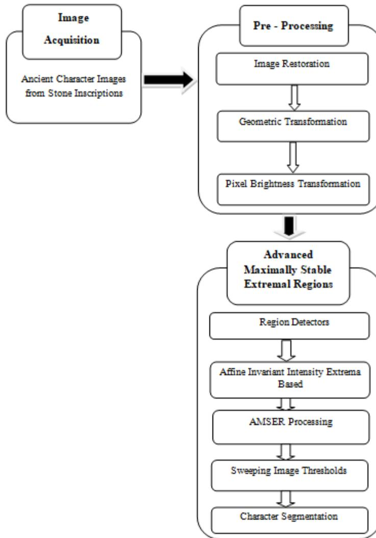
Figure 3: Architecture for Character recognition using AMSER Algorithm
