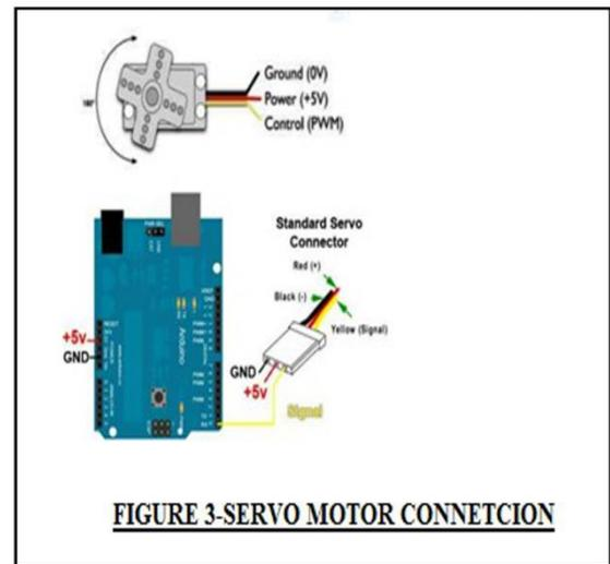
Figure 3: Servo motor configuration
