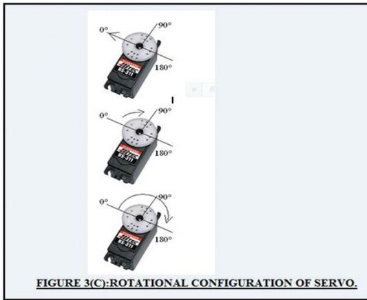
Figure 5: Rotational configuration of servo
