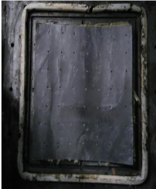
Fig.2 Stacking of drilled Al/Fibres in Die
