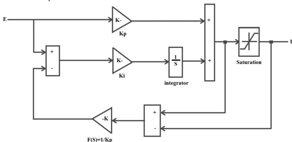
Figure 2. Simulation diagram of Anti Wind up PI controller
