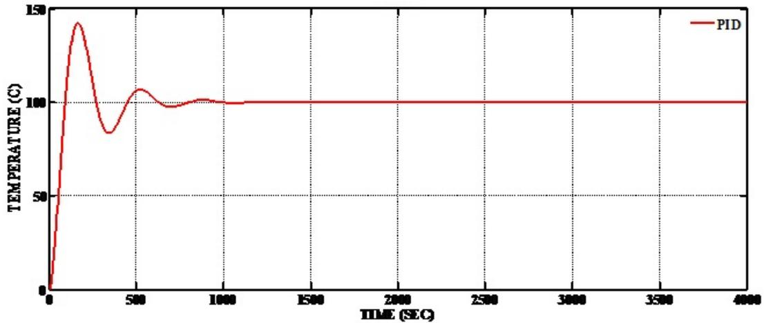
Figure 5. Temperature of PID controlled extrusion system
