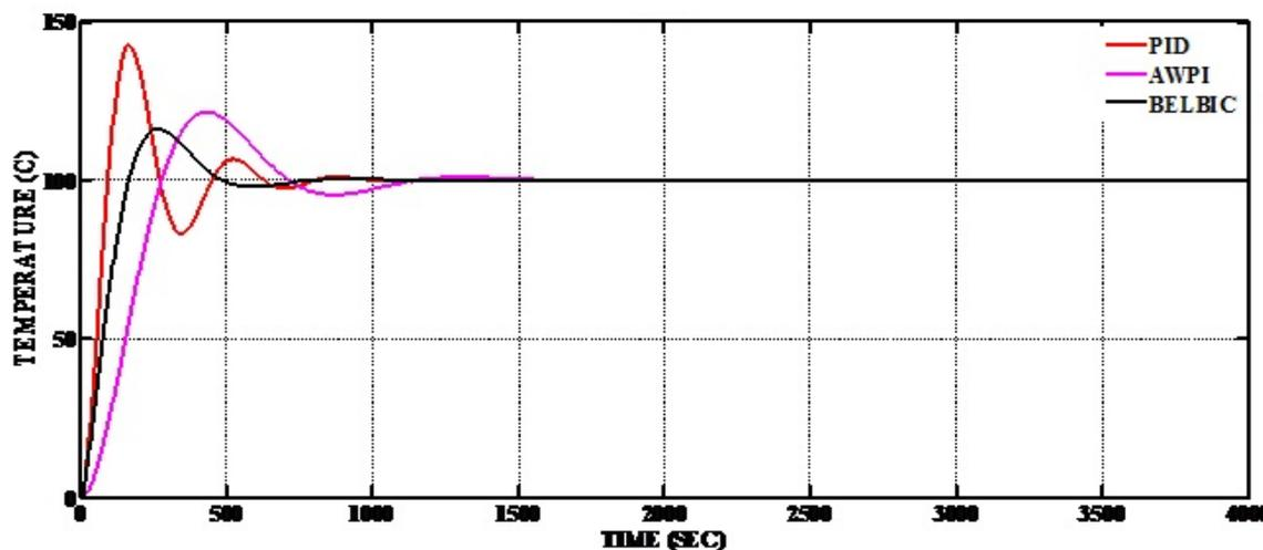
Figure 8. Comparison of PID, AWPI and BELBIC in extrusion control
