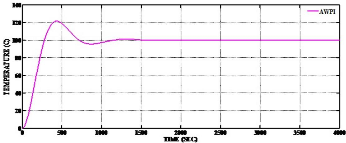
Figure 6. Temperature of AWPI controlled extrusion system
