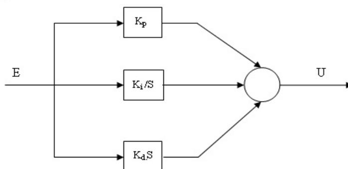
Figure 1. Block diagram of PID controller
