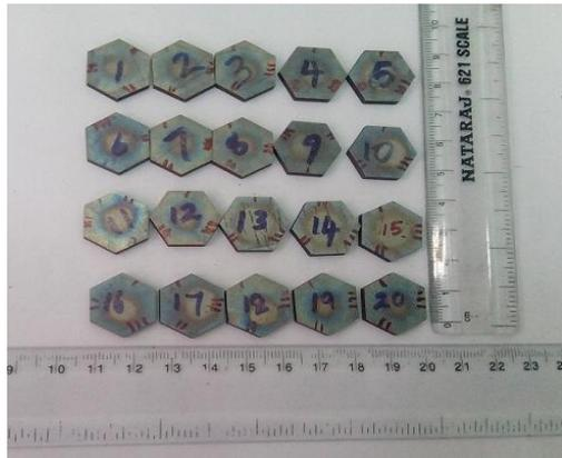
**Figure 3 Machined Samples of Ti Grade 2(Brass wire)**
