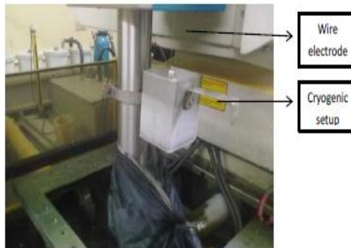
**Figure 2 Cryogenic setup mounted on WEDM machine**
