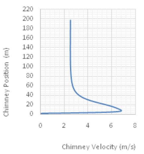
Fig 9: Plot of Velocity along the length chimney for Spanish Model
