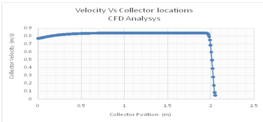
Fig 12: Plot of Velocity along with the collector (Experimental Model)
