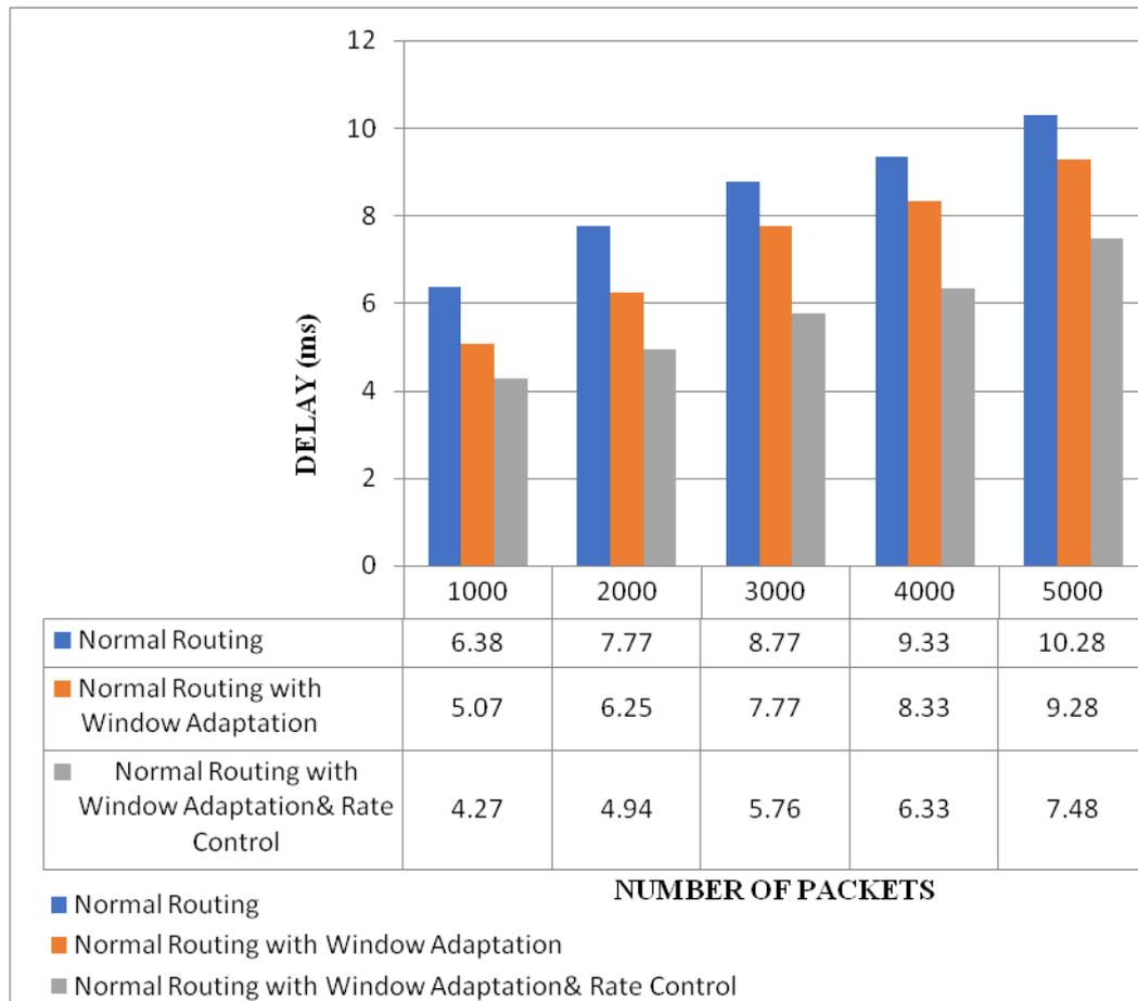
**Fig. 6 Delay Vs Number of Packets**
