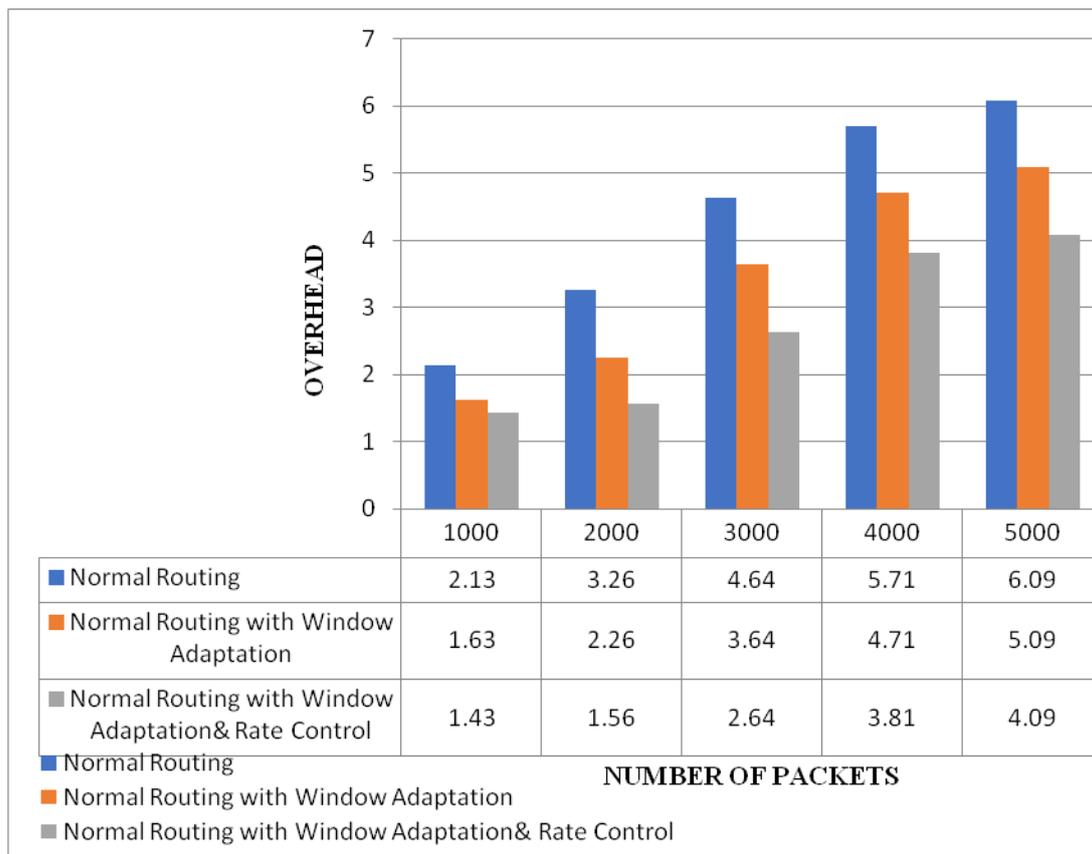
**Fig. 5 Overhead Vs Number of Packets**
