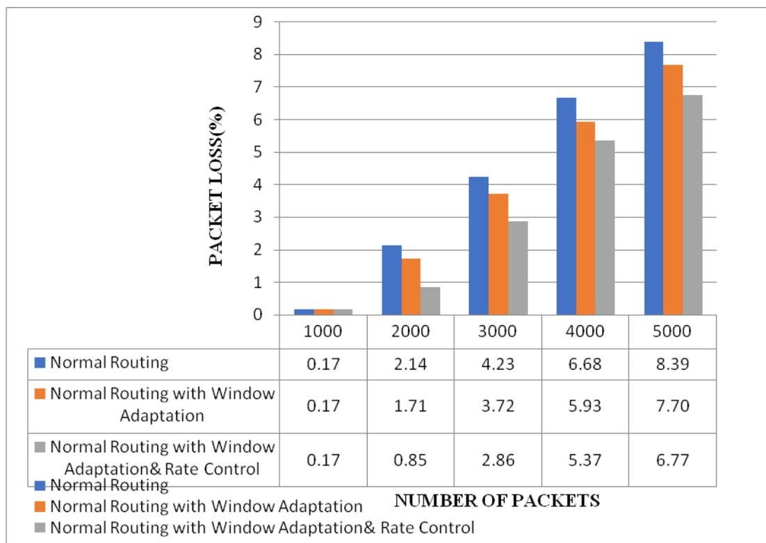
**Fig. 4 Packet loss Vs Number of Packets**
