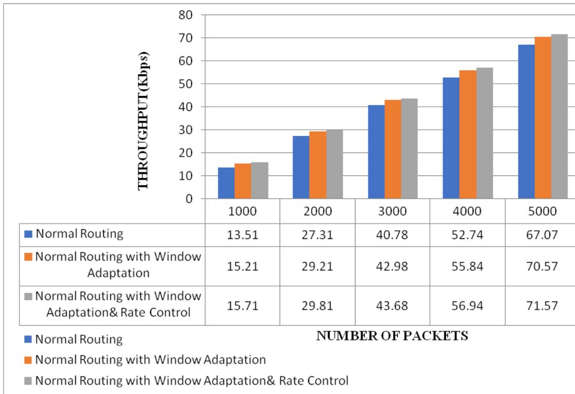
**Fig.7 Throughput Vs Number of Packets**
