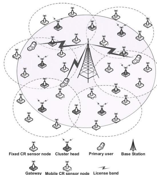
**Fig. 1 System Architecture for CRSN**
